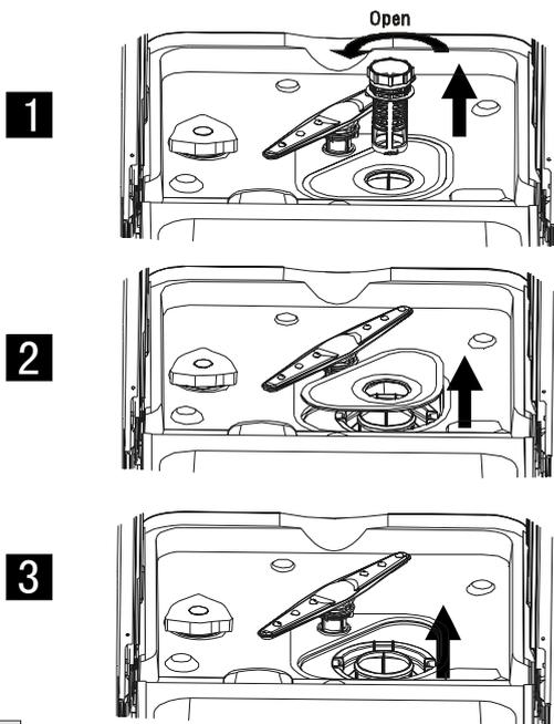
Step 1 : turn the filter cylinder counter-clockwise, then lift it up
