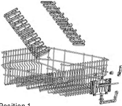
\*\*\*NOTE\*\*\*: The upper rack has side flaps (pictured at left Above basket). There are 4 (2 on each side). These can be Adjusted into 2 positions = position 1 (high) and position 2 (low).
