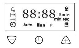
Touchpad SET(-): Conductive key fitted into Touchpad position 1 or 2 Touchpad SELECT: Conductive key fitted into Touchpad position 3 Touchpad SET(+):Conductive key fitted into Touchpad position 4 or 5
