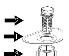
The filter system consists of a coarse filter, a flat (Main filter) And a microfilter (Fine filter).
